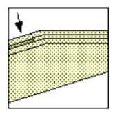
4. Attach fin spar and ensure fin spar angle is  $15^{\circ} \pm 1^{\circ}$ . Attach the fin spar opposite the vent hole with white glue.
