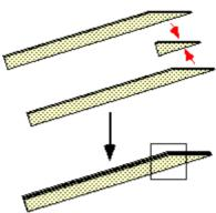
Note that there should be a space between the fin spars (see enlarged detail). This gap will later be used to hold the fin.
